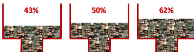
Figure 2. Used percentages of the forwarder load capacity in case of: conventional treatment (on the left), load compression (in the middle), and rough-delimiting (on the right).
