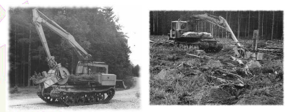
Container seedling planting machine "KLM-1" (Russia) mounted on excavator "TB-1" able to make mound and simultaneously plant seedling on it 1983.
