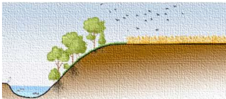
Figure 11 Very steep slope, “run offs washout tolerant” grass stripe (~2m) and mixed tree going to establish “multi-layer roots net” (modified E. Hodgson, 2023).
