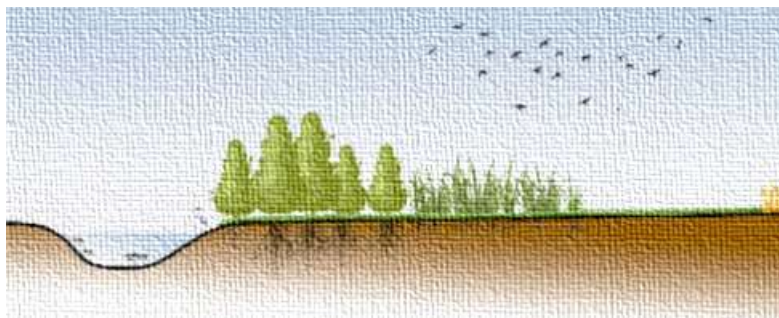
Figure 6. CRC SRF 20 combine buffer - where 5-7m wide Populus spp. planted next to Salix spp. or reed canary grass 5-7 m. Between cropland and trees at least 6-meter-wide undisturbed technical corridor (modified E. Hodgson, 2023).
