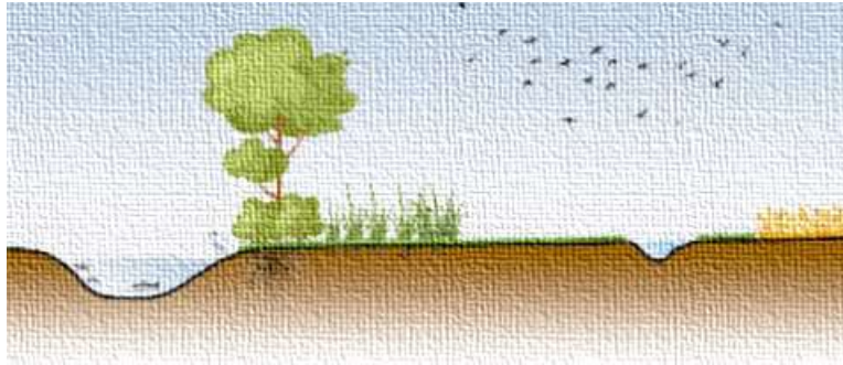
Figure 7 Coppice standards (3m wide zigzag row (with low bush or perennial grass stripe (5-7m), undisturbed technical corridor (~6m) and shallow accumulating ditch (modified E. Hodgson, 2023).
