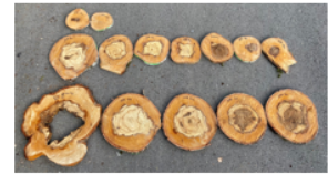
Cross-section discs of birch with stem rot
