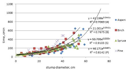
Figure 2. Productivity of stump extraction depending on dimensions of stumps.
