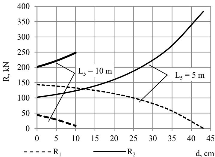
**Fig. 2.3. The diameter of stumps ( $d$ , cm) and influence of hydraulic manipulator ( $L_5$ ) boom on response to support of tracks**
