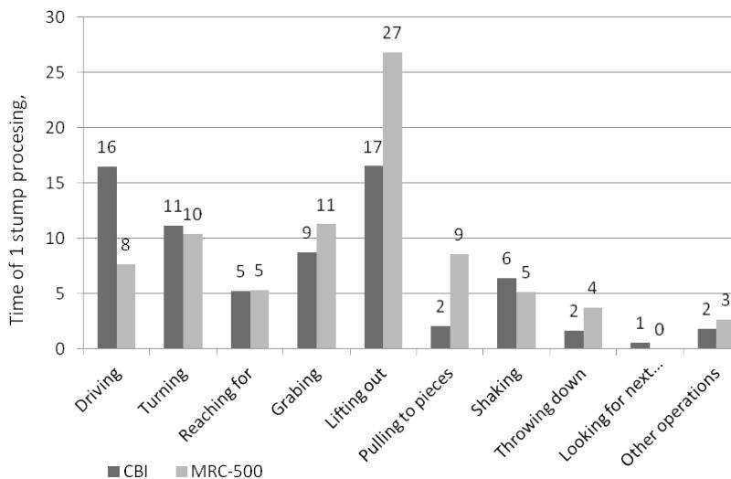
Figure 1. Comparison of structure of productive time consumption.
