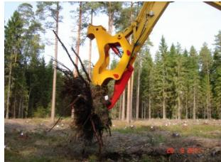
Figure 3. Stump extraction MCR 500.
