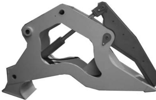
Figure 1. Stump lifting head MCR-500.
