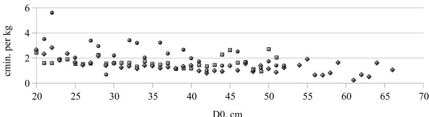
Figure 2. Productivity of stump extraction depending on dimensions of stumps.
