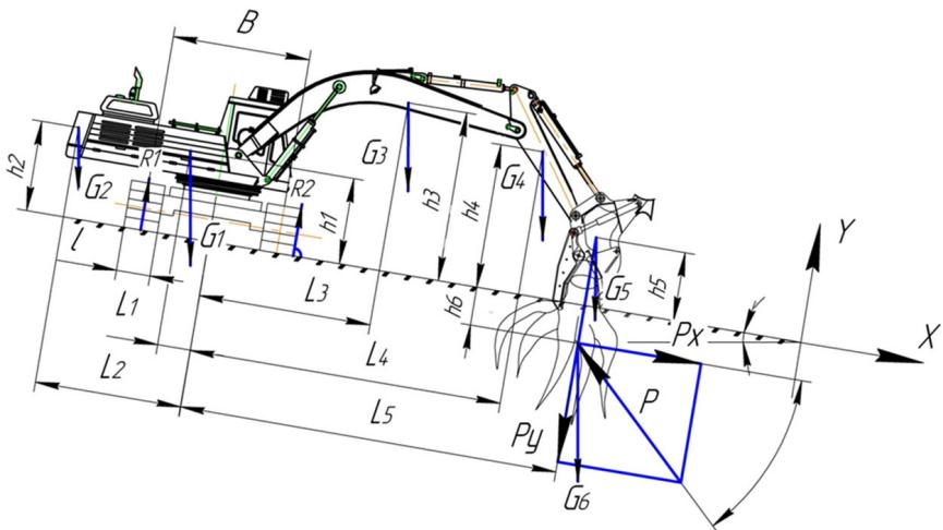
**Fig. 2.2. Force calculations for stump extraction**
