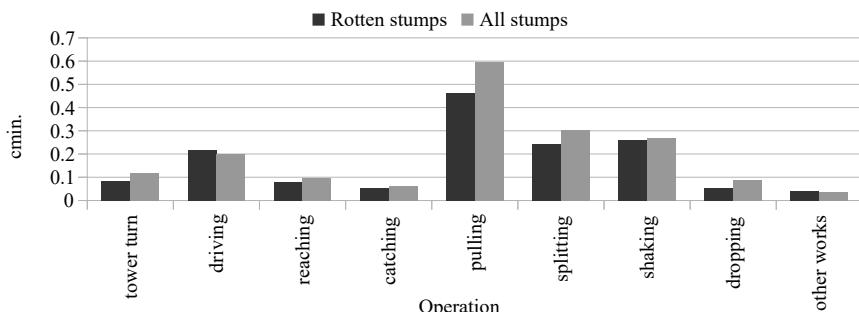
Figure 3. Productivity of extraction of rotten stumps – comparison of work elements.
