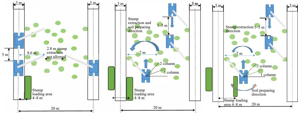
**Fig. 2.1. Work methods for stump-pulling**
