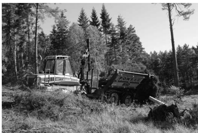
Figure 1. The forwarder had dedicated residue load area.
