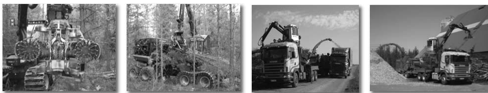
Figure 1. A conventional harvester head equipped with multi-tree-handling accessories (left) and Fixteri II bundle harvester. Chipping of energy wood at a roadside landing or at a terminal using a trailer-mounted drum chipper (right).
