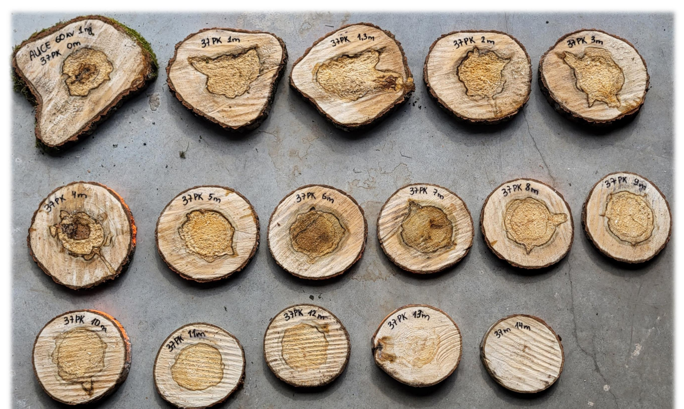
Determining the prevalence of internal stem decay by the cross-section discs.
